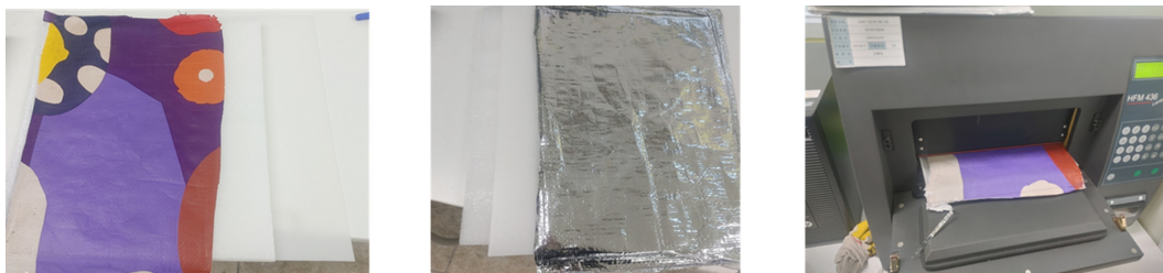
Fig. 2. Measurement of Thermal Conductivity for EPE Boxes.
