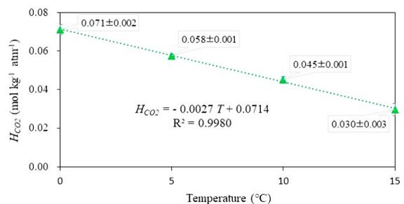
**Fig. 1.** H<sub>CO<sub>2</sub></sub> (CO<sub>2</sub> solubility) of rockfish fillet as function of temperature. Vertical bars are standard deviations
