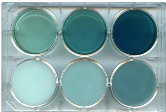
Fig. 3. The color changes over time (from left to right) of the original TTI (top row) and new improved TTI (bottom row).
