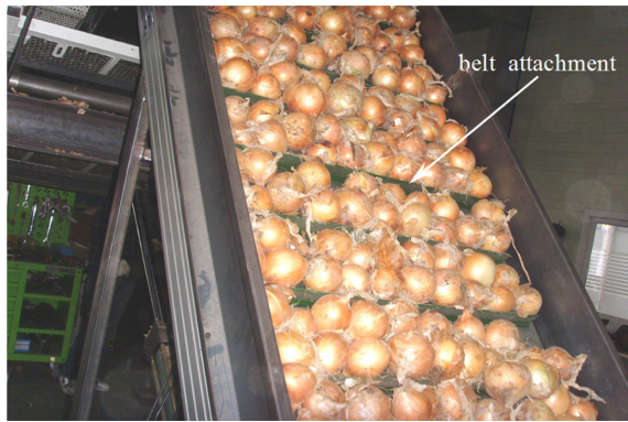
Fig. 7. View of measuring test of area rate occupied by onions of inclined belt conveyor.
