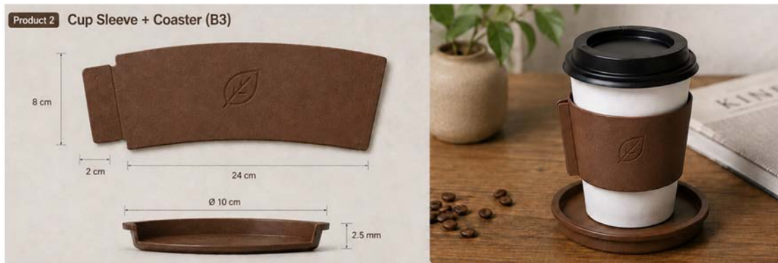
Fig. 16. Cup sleeve and coaster set (B3 formulation) design: sleeve flat pattern (24 × 8 cm), coaster (Ø 10 cm), and coaster cross-section detail.
