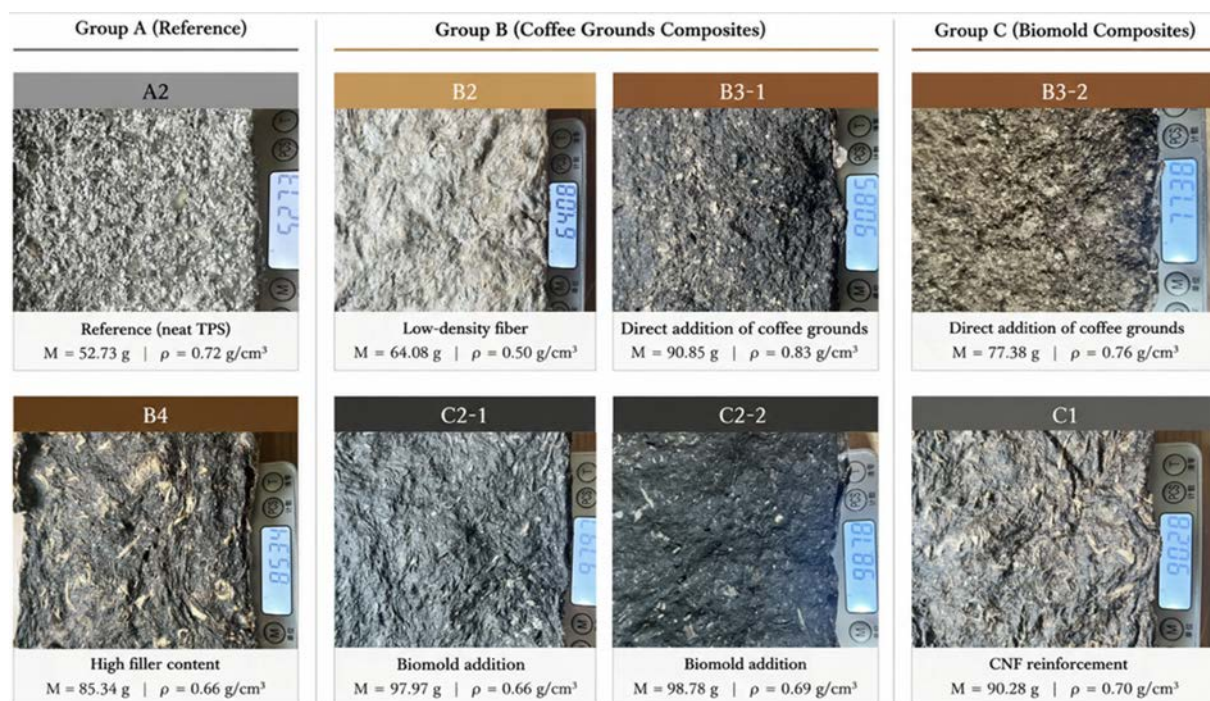
Fig. 2. Appearance of fabricated composite specimens for each sample group.
