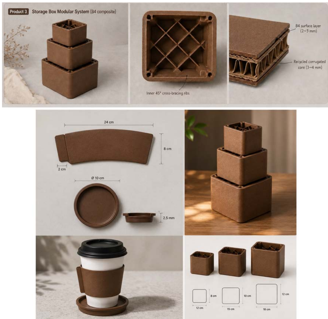
Fig. 19. Modular storage box (B4 composite formulation) design: three-module set (S/M/L), 45° internal lattice ribs, and composite cross-section (B4 skin 2-3 mm + recycled corrugated core 3-4 mm).
