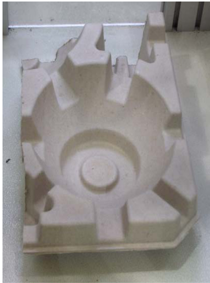
Fig. 3. 1/4 sample for shock absorbing test.
