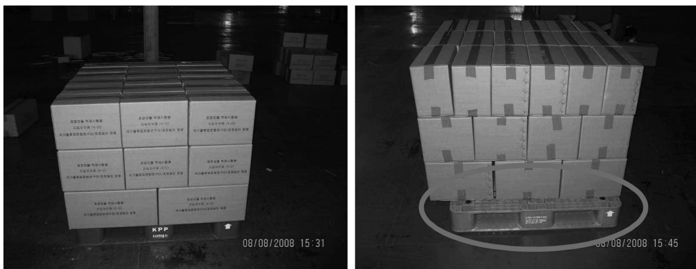
Fig. 4. Stacking patterns of K-type packaging module (Left pallet: 1,100 × 1,100 mm, Right pallet: 1,200 × 1,000 mm)
