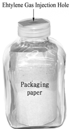
Fig. 1. Test bottle used for determining the adsorption efficiency of ethylene gas of packaging paper.
